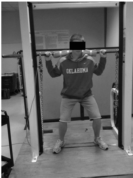
Figure 3. Front view of isometric squat test set up with heels positioned over marker 1, feet shoulder width apart and Knee joint angle standardized to 135^{\circ} \pm 5^{\circ} .
